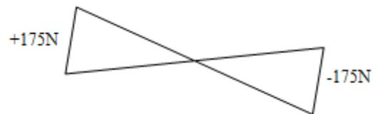
Fig. 4: Shear force diagram for side AB
