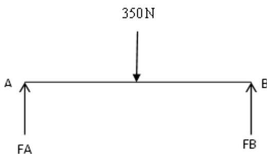
Fig. 2: Modified Free Body Diagram for side AB condition for equilibrium
