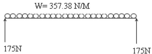
Fig. 3: Body Diagram of the Bed frame
