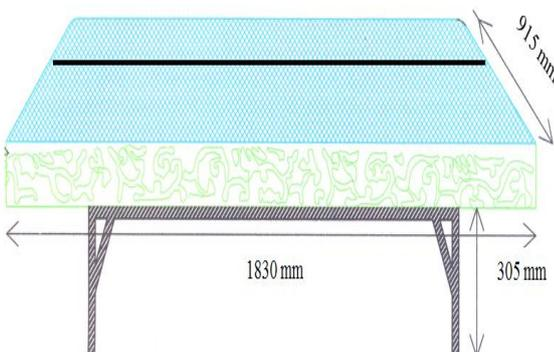
Fig.8: Fabricated Chair- Bed in Bed Form
