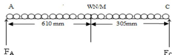
Fig.1: Free-body diagram for side AB
