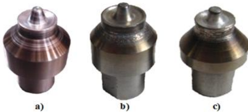
Fig.1 Welding tools used for welding AZ 31B with pin inclination a) 20°; b) 15°; c) 6°
