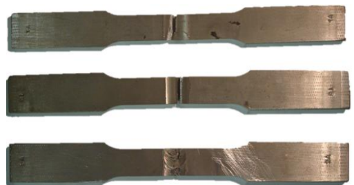
Fig. 6 Specimens after destruction of welded joint
