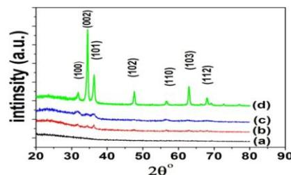
**Fig. 1. (a, b,c & d) XRD of ZnO nano-particles (seed layer) before the growth of (NRs) prepared by spin coating sol gel method, heated at different temperature 100 (a), 150 (b), 250°C (c), respectively. typical XRD of ZnO (NRs) prepared by aqueous chemical growth at 90°C (d)**
