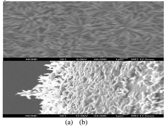
Fig. 6. Typical scanning electron microscopy (SEM) images of ZnO nano-rods grown on gold coated glass substrate (a) before coating with iron membrane, (b) after coating with iron membrane.
