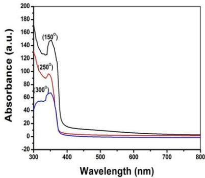
Fig.8. The absorbance of the ZnO (NRs) prepared at different temperature 150, 250 and 300°C prepared by (ACG).
