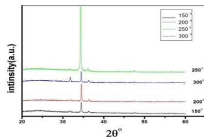
**Fig. 2. XRD patterns of the ZnO NRs thin films prepared on seed layers under different annealing temperatures.**
