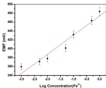
Fig. 11. Calibration curve of the electrochemical potential difference, for the gold coated glass substrate ZnO (NRs) as potentiometric electrode with Ag/AgCl reference electrode versus Logarithmic concentration range for  $Fe^{3+}$  change for buffer solution.
