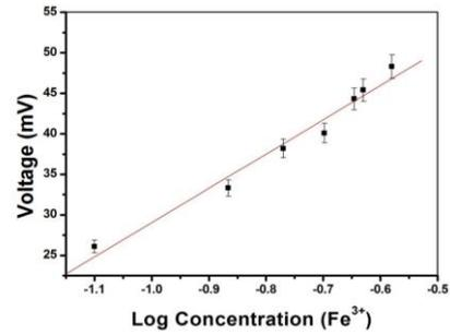
Fig. 12. Calibration curve of the electrochemical potential difference, for gold coated glass substrate ZnO (NRs) as potentiometric electrode with Ag/AgCl reference electrode versus Logarithmic concentration range for  $Fe^{3+}$  change for Hemoglobin solution.
