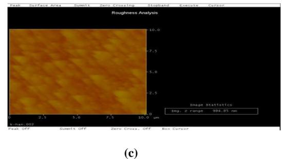
Fig.7. AFM images of ZnO (NRs) prepared by low temperature (ACG) method.
