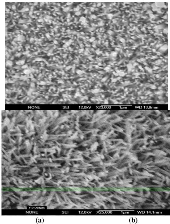
Fig.5. Typical scanning electron microscopy (SEM) images of ZnO nano-rods grown on glass substrate, with seed layers at annealing temperature 300<sup>o</sup> C (a) 3 layers (b) 6 layers.
