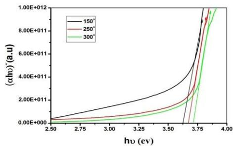
Fig.10.  $(\alpha h\nu)^2$  as a function of photon energy for the ZnO nanorod thin films annealed at different temperature at 150, 250 and 300°C, respectively.
