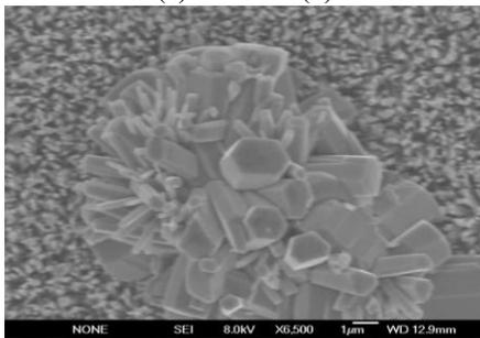
Fig.4. Typical scanning electron microscopy (SEM) images of ZnO nano-rods grown on glass substrate, with seed layers at annealing temperature 250<sup>o</sup> C (a) 3 layers (b) 6 layers and (c) 6 layers to focus on the hexagonal structure.
