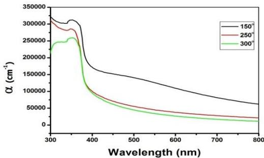
Fig.9. The absorption coefficient ( $\alpha$ ) of ZnO (NRs) prepared at 3 different temperature 150, 250 and 300°C by (ACG).
