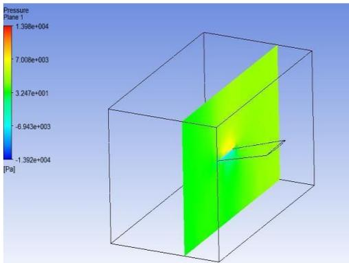
Fig. 11. Plane located on wall-solid showing pressure distribution
