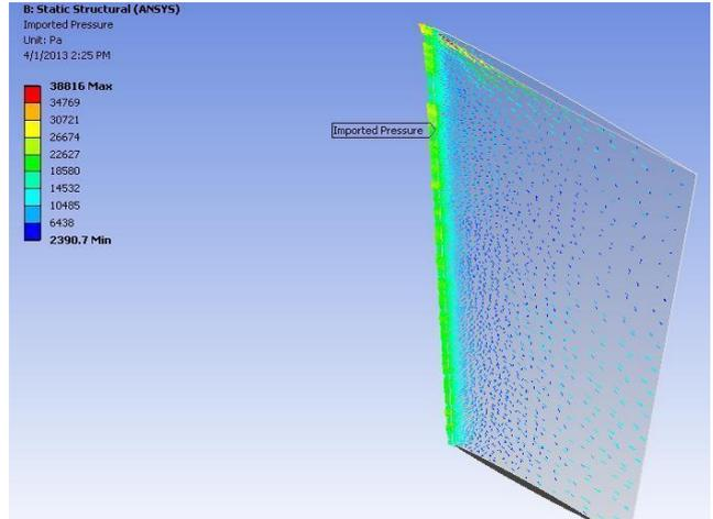
Fig. 14. Showing imported pressure acting on a wing.
