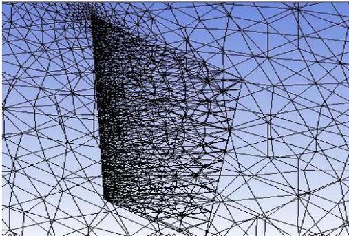
**Fig. 7. Showing mesh over the wing for the CFD Analysis using wireframe view**
