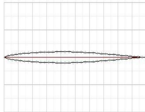
Fig. 2. Airfoil generated using Foilsim software
