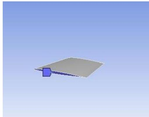
**Fig. 9. Fixed support applied at root chord of the wing**
