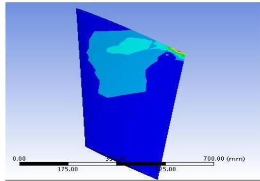
Fig. 15. Contour of total deformation on wing
