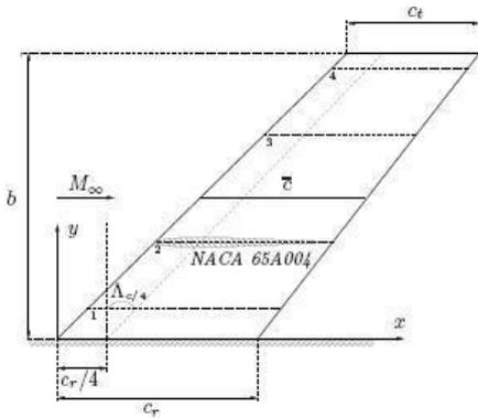
Fig. 3. AGARD 445.6 wing model (with reference to Ramjikamakoti thesis)
