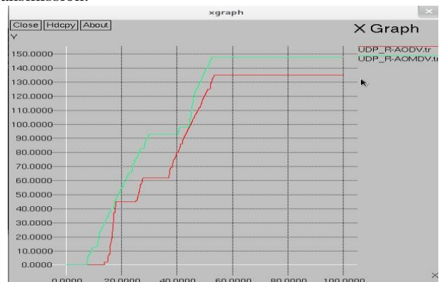
Fig 4: UDP Packets Receive Analysis For AODV and AOMDV
