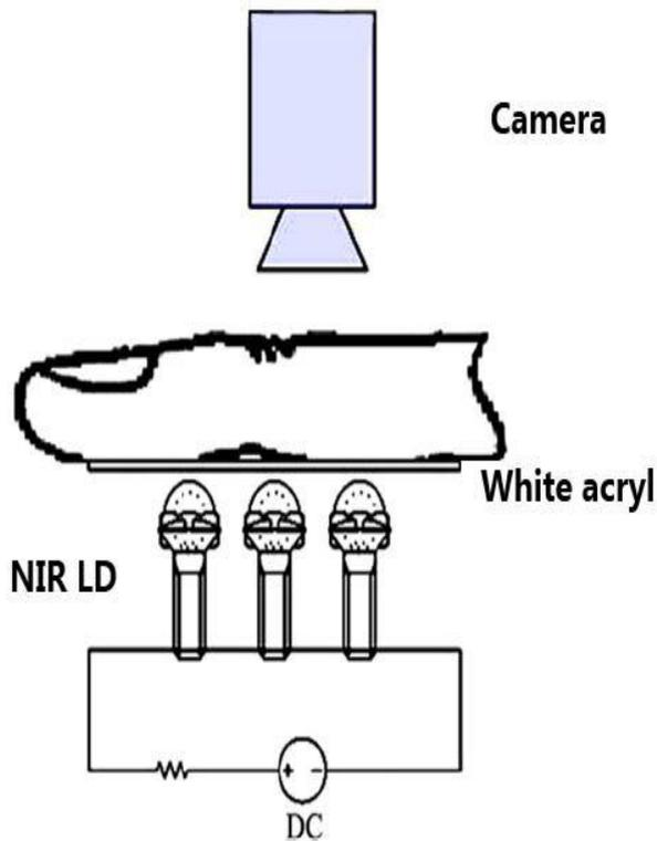
**Fig.3. The illustration of the imaging device**
