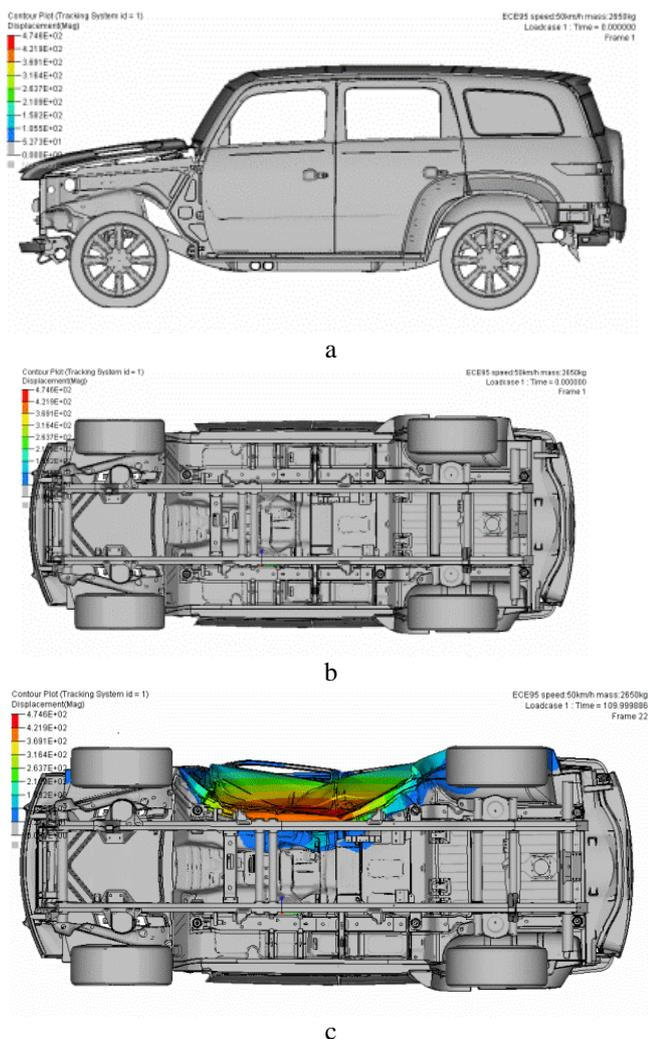
Fig 2 Results of Side impact test, a)tracing displacement side view, b) bottom view, middle left, c) bottom view results for front, medium, right part of crash zone, exaggerated
