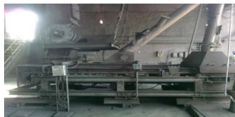
Weigh feeder for sending the fine coal to preheater and kiln Flow diagram coal grinding:
