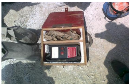
Equipment used for blasting ( dc battery)
