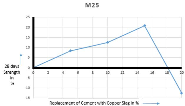
Fig 3: Variation of split tensile strength w.r.t. the variation of % of copper slag in M25
