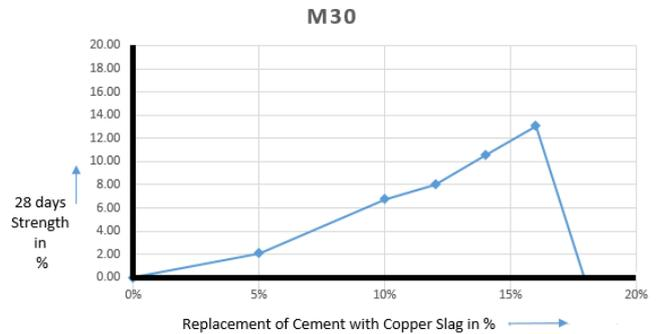
Fig 2: Variation of compressive strength w.r.t. the variation of % of copper slag in M30
