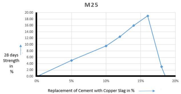
Fig 1: Variation of compressive strength w.r.t. the variation of % of copper slag in M25
