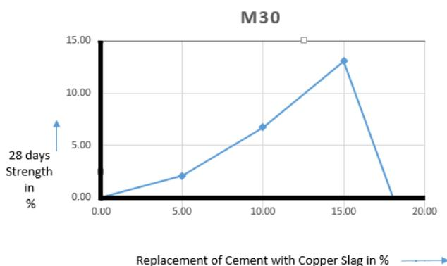
Fig 6: Variation of flexural strength wrt the variation of % of copper slag in M30
