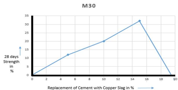
Fig 4: Variation of split tensile strength w.r.t. the variation of % of copper slag in M30
