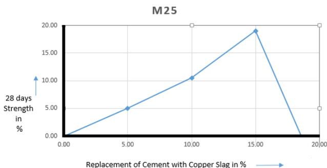
Fig 5: Variation of flexural strength w.r.t. the variation of % of copper slag in M25
