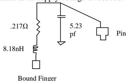
Fig 11. DIP-40 package pin ground bounce noise model
