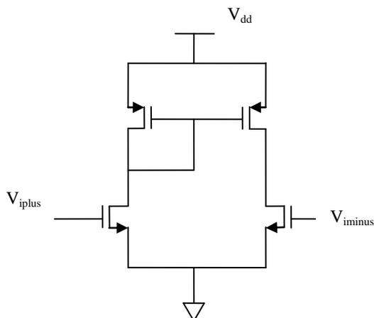
Fig 5. Schematic of comparator
