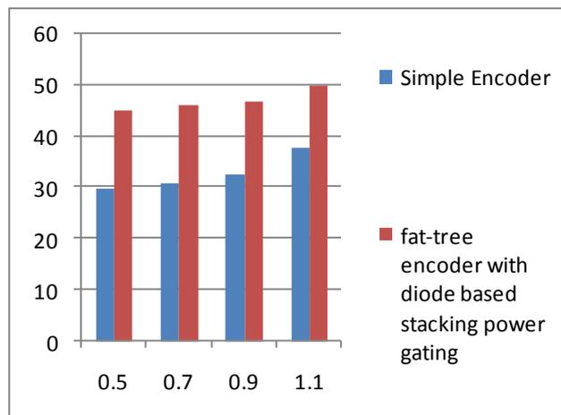
**Fig 9. Active Power Dissipation of Fat-tree encoder**
