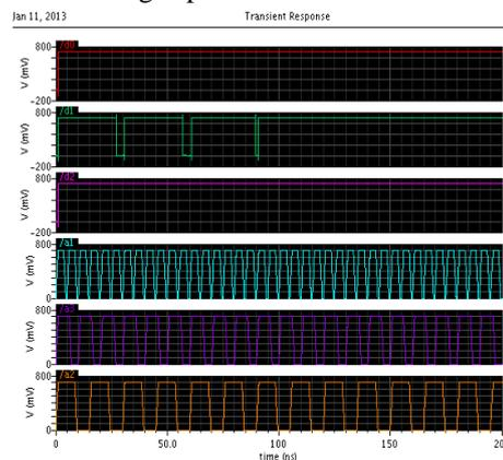
Fig 4. Transient Response of Fat-tree encoder
