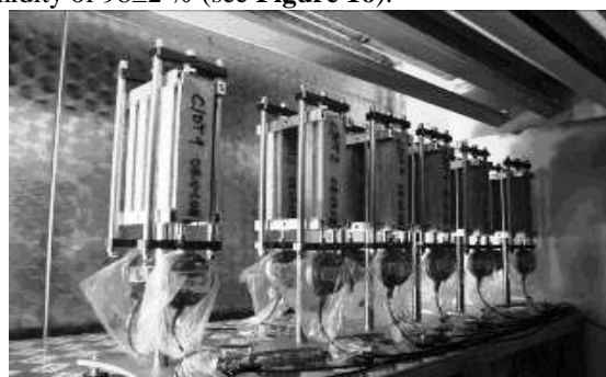
Fig 16. Apparatus for the measurement of expansion of hardened concrete according to ASTM C490-86 placed in a climatic chamber.
