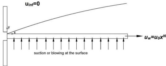
Fig 1. Schematic of permeable stretching surface
