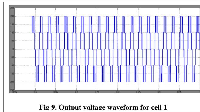
Fig 9. Output voltage waveform for cell 1
