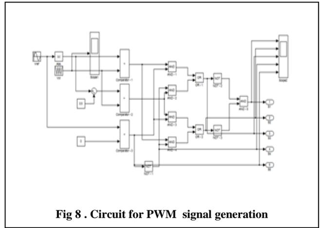
Fig 8 . Circuit for PWM signal generation
