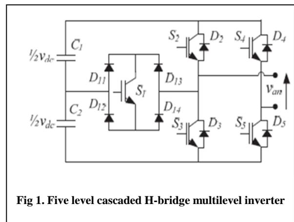
Fig 1. Five level cascaded H-bridge multilevel inverter
