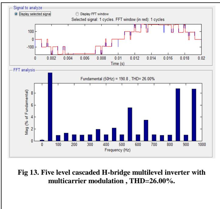
Fig 13. Five level cascaded H-bridge multilevel inverter with multicarrier modulation , THD=26.00%.
