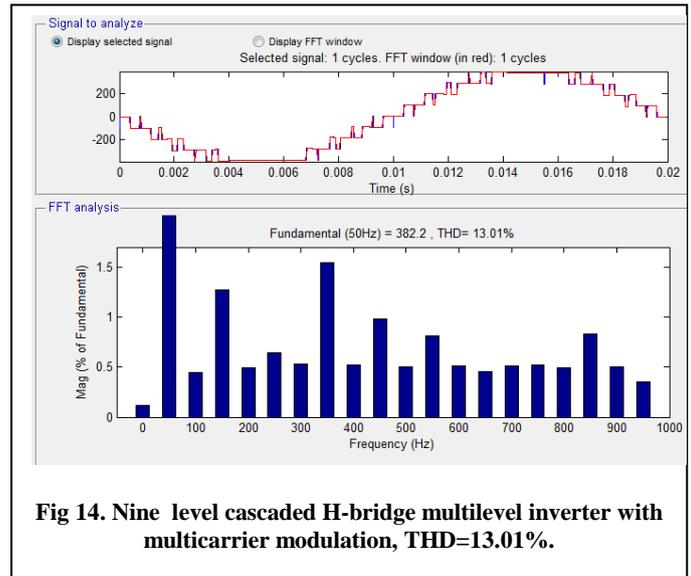
Fig 14. Nine level cascaded H-bridge multilevel inverter with multicarrier modulation, THD=13.01%.
