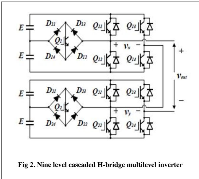
Fig 2. Nine level cascaded H-bridge multilevel inverter
