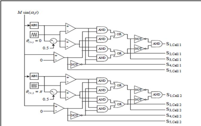
Fig 4. PWM signal generation with multicarrier phase-shifted modulation
