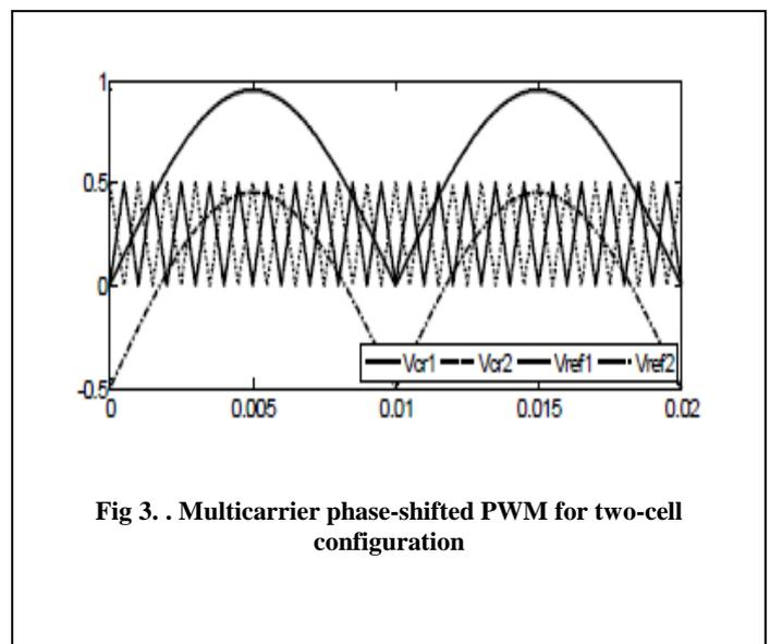
Fig 3. . Multicarrier phase-shifted PWM for two-cell configuration
