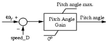
Fig 10: Pitch angle control method [5]
