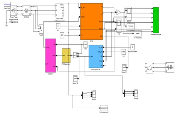
Fig 3 Simulink model for DFIG(Rotor Side)
