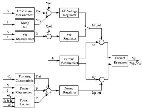
Fig 2 Rotor converter control block diagram[2]
