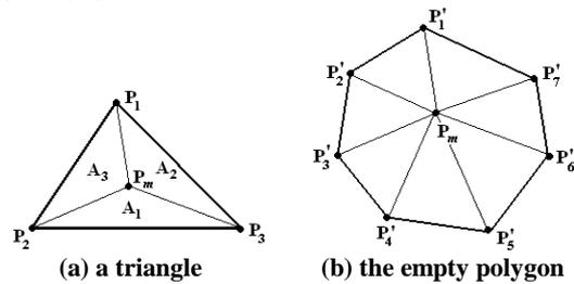
Fig. 6. Insertion of interior point
