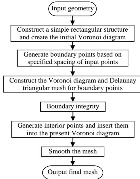
Fig. 1. The procedures of Delaunay triangulation
