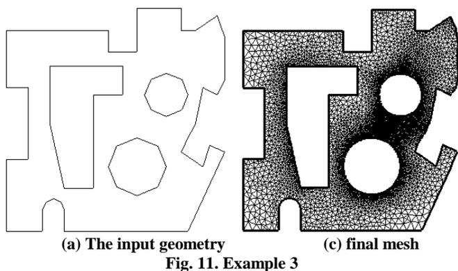
(2) Our system resolved boundary loss problem by adding pseudo-points. Two criteria for selecting removal modes were employed as well. By using this method, the lost boundaries are recovered successfully. The mesh after boundary integrity can capture the boundary features of the geometry accurately.
