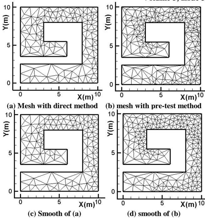
Fig. 7. Insertion and smooth of interior nodes
