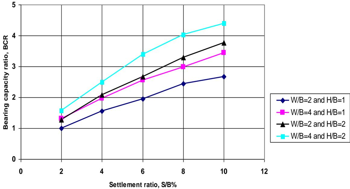
Fig. (9) BCR variation with settlement of footing for various H/B and W/B ratios
