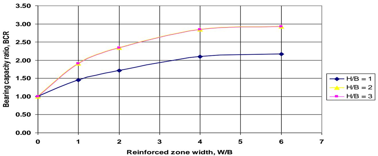
Fig. ( 8 ) Effect of reinforced zone width ( W/B ) on bearing capacity ratio BCR
