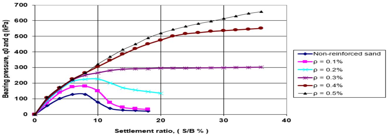
Fig. (10) Pressure-settlement relationships for different fiber concentration with ( H/B= 3 and W/B = 2 )
