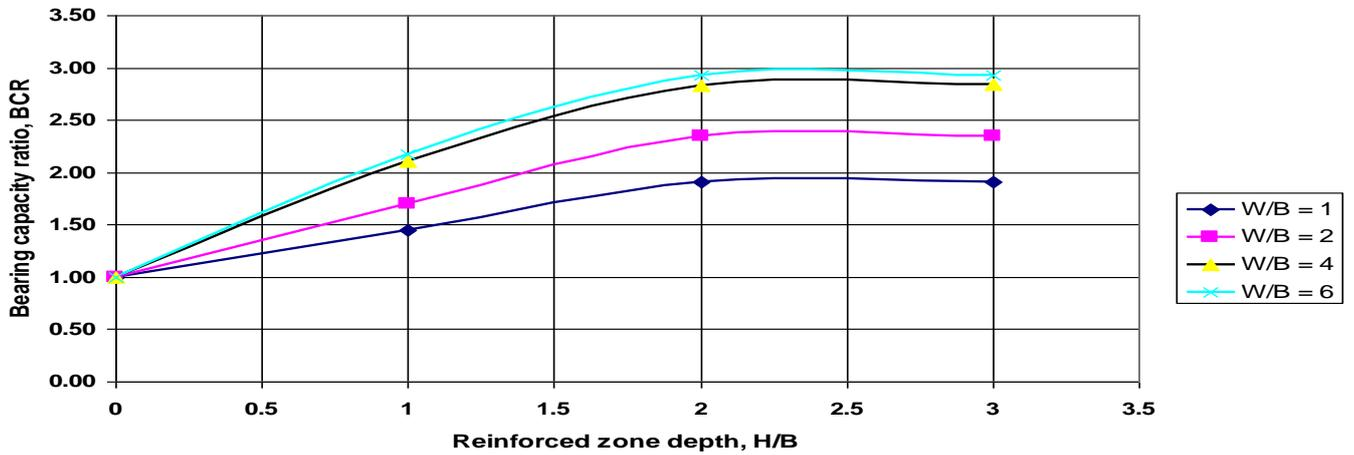
Fig. ( 7 ) Effect of reinforced zone depth H/B on bearing capacity ratio BCR
