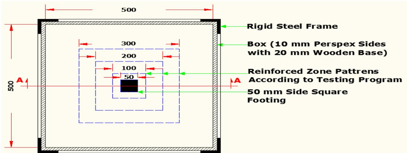
**Fig. (1) Model Test Plan**
