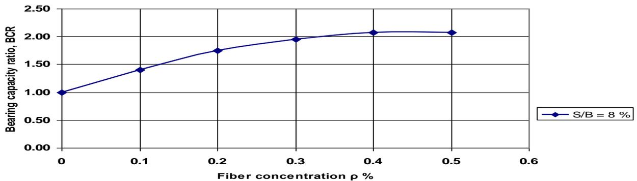
Fig. (11) Effect of fiber concentration  $\rho$  % on bearing capacity ratio BCR
