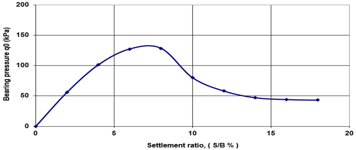
Fig. ( 3 ) Pressure - settlement relationship for non-reinforced
