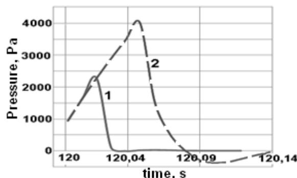
Fig. 9. Pressure Curve at Ignition on the 120<sup>th</sup> Second at Operation of Various SS: 1-Wall; 2-Window
