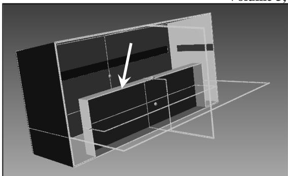
Fig. 4. Internal Close-Spaced Volume in FV Model, Simulating Equipment
