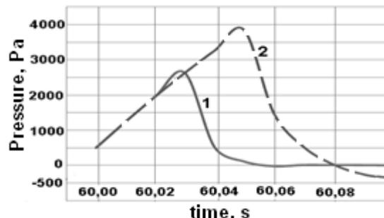
Fig. 8. Pressure Curve at Ignition on the 60<sup>th</sup> Second at Operation of Various SS: 1-Wall; 2-Window
