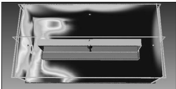
Fig. 6. Mix of Gas and Air in a Shop with Defective Pipelines
