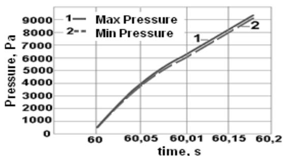
Fig. 7. Pressure Curve at Ignition on the 60<sup>th</sup> Second and Nonoperation of Any Type of SS
