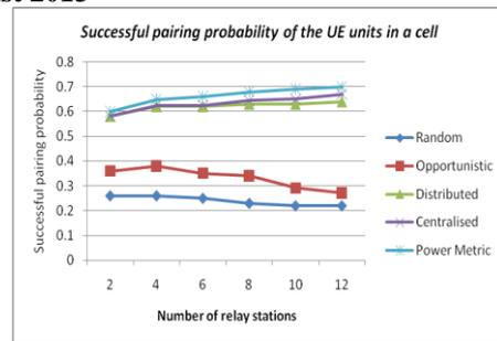
Fig 4 : Successful pairing probability of the UE units in a cell.
