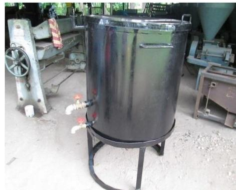
Plate 1. Constructed Local Improved rice Parboiler
