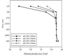
Fig. 10b Comparison of maximum tensile stress for different spans subject to 5 kN load
