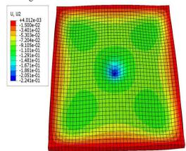
Fig 6: Deflection contour of funicular shell of span 1m with span to rise ratio of 20
