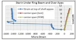
Fig.12 Comparison of maximum compression and maximum tension
