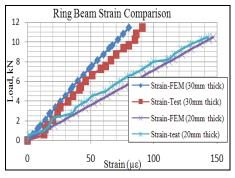
Fig.14 comparison of tensile strain at centre span of ring beam
