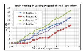
Fig.11 Comparison of load and strain at leading diagonal top surface of 20mm thick shell
