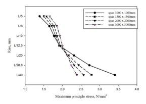
Fig. 10a Comparison of maximum tensile stress for different spans subject to 2.5 kN load
