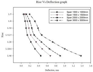
Fig. 8a Comparison of maximum deflection for different spans subject to 2.5KN load
