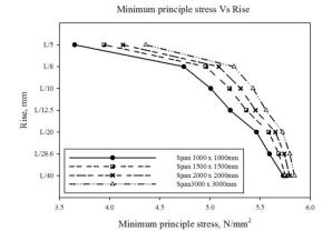
Fig. 9a Comparison of maximum compressive stress for different spans with 2.5 kN load
