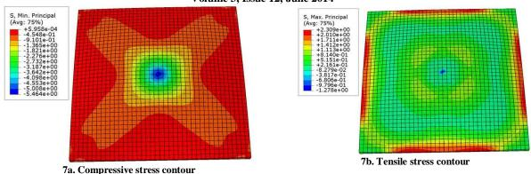
Fig. 7 Typical stress contour for funicular shell of 1m span
