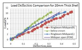
Fig.13 Deflection Comparison of 20mm thick shell
