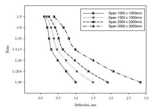
Fig. 8b Comparison of maximum deflection for different spans of shell with 5 kN Load
