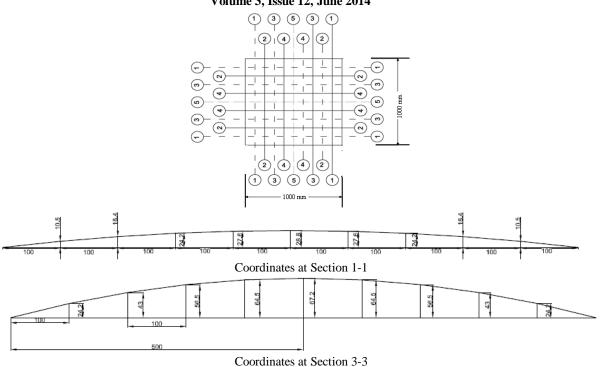
Fig.1 Coordinate development for shell form generation
