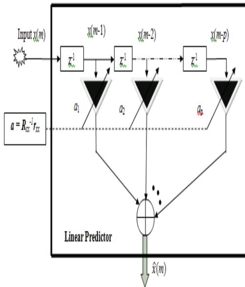
Fig. 1 Diagram of the Linear Predictor
