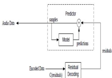
Fig. 3 Decoding Process
