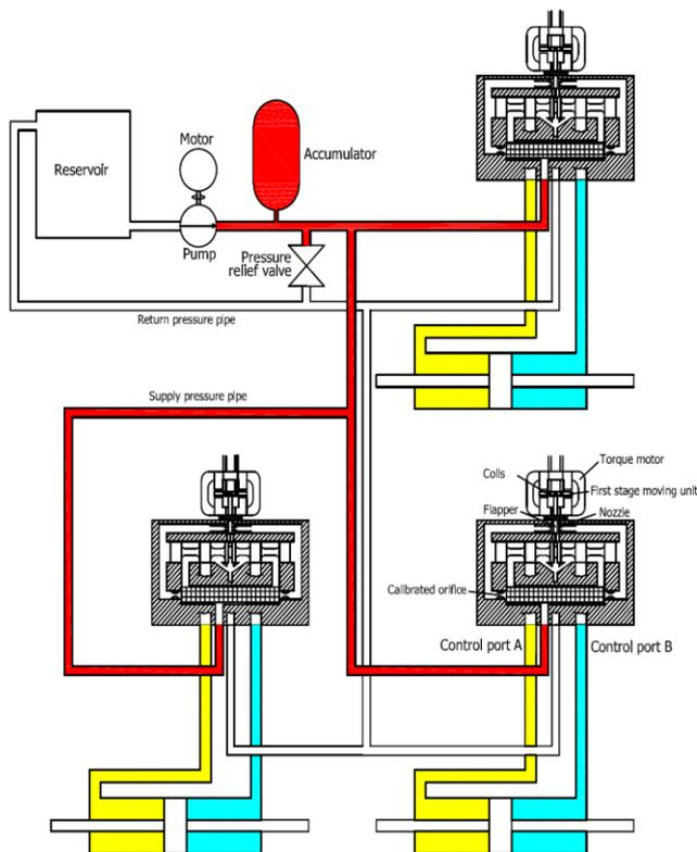
Fig 1. Schematic of the hydraulic system and related users.
