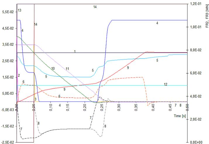
**Fig 7. Actuation with users 2 and 3 equipped with reduced spool stroke (67% of the stroke in opposing load condition).**
