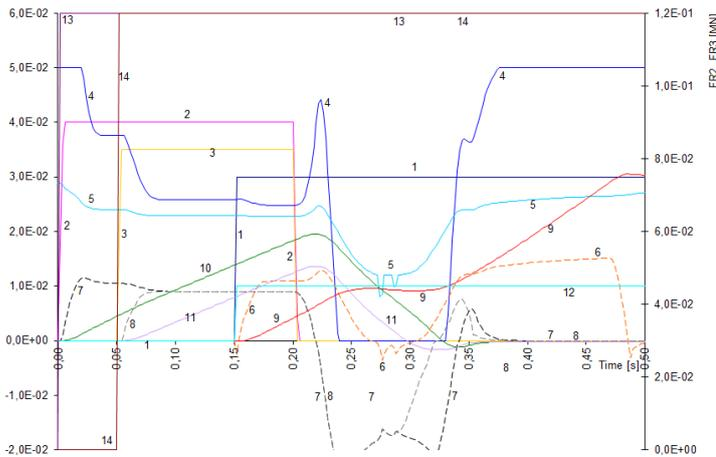
**Fig 14. Actuation with users 2 and 3 equipped with reduced spool stroke (83% of the stroke in opposing) – quick motion reversion commanded.**
