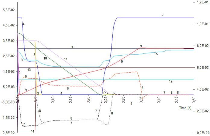
**Fig 11. Actuation with users 2 and 3 equipped with reduced spool stroke (67% of the stroke in opposing load condition) and with loads of 60 kN.**
