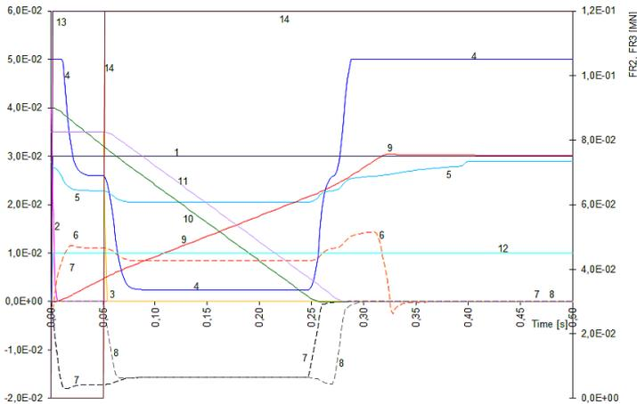
**Fig 8. Actuation with users 2 and 3 equipped with reduced spool stroke (50% of the stroke in opposing load condition).**
