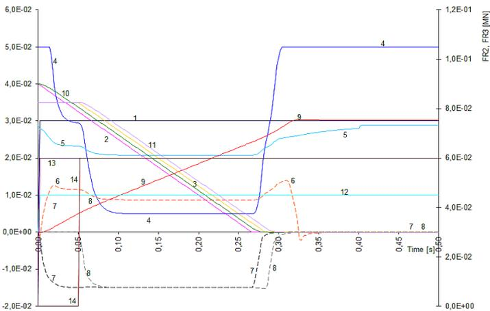
**Fig 9. Actuation with users 2 and 3 equipped with a ramp generator and with loads of 60 kN.**
