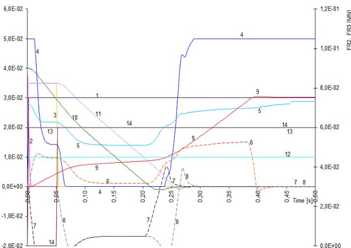
**Fig 10. Actuation with users 2 and 3 equipped with reduced spool stroke (83% of the stroke in opposing load condition) and with loads of 60 kN.**
