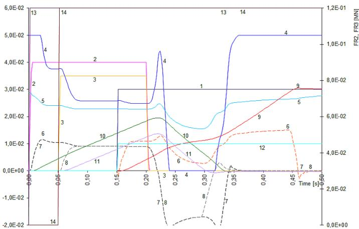
**Fig 15. Actuation with users 2 and 3 equipped with reduced spool stroke (67% of the stroke in opposing) – quick motion reversion commanded.**
