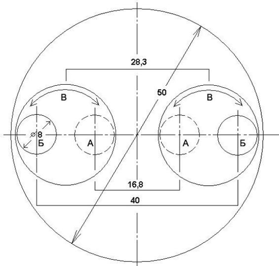
**Fig. 3. Chart of 2-channel SQUID-Magnetometer with a Variable Base.**
