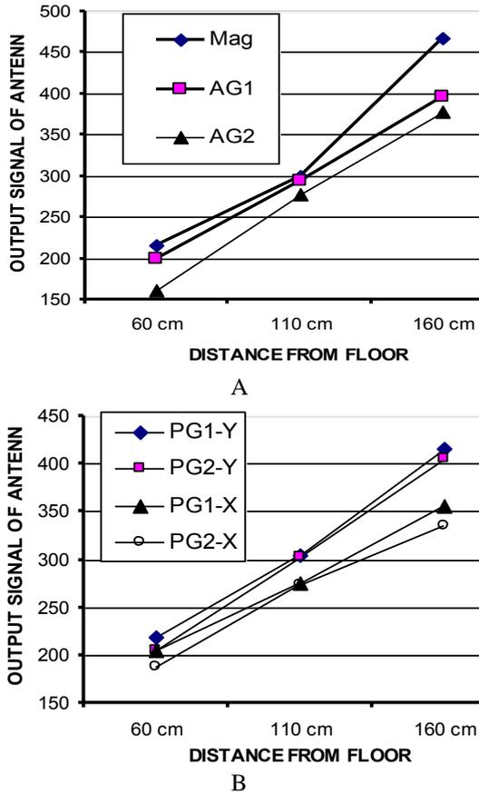
Fig. 1. Dependence of magnetic disturbances from distances to floor: a – axial, b - planar antennas.
