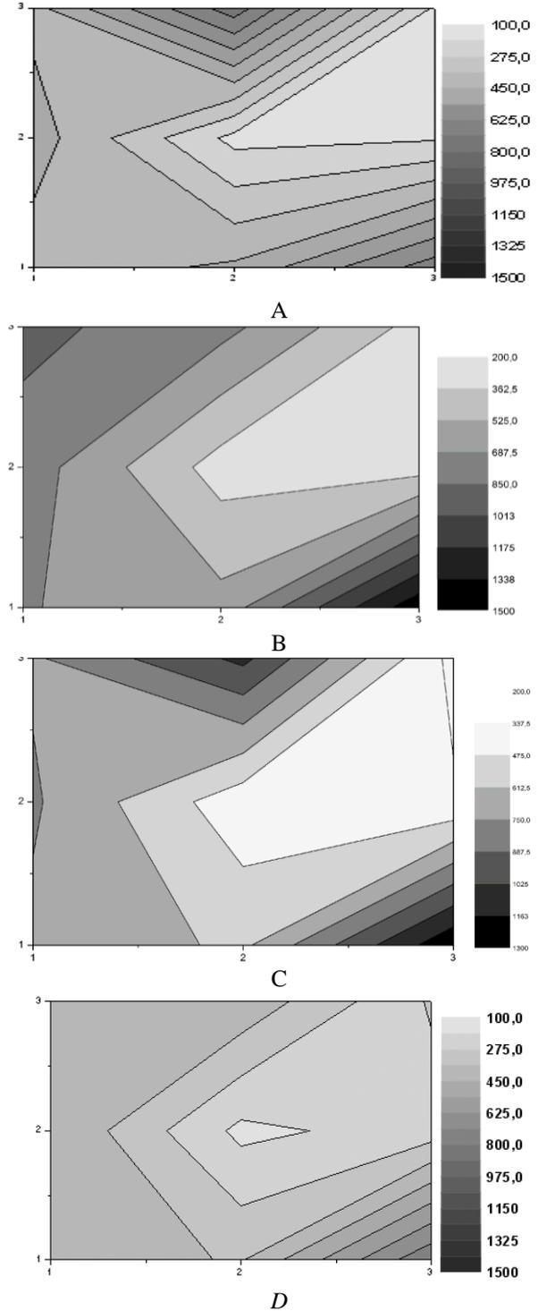
Fig. 2. Distribution of disturbances at lab room: magnetic field (A), 1<sup>st</sup> (B), 2<sup>nd</sup> (C), vertical 2<sup>nd</sup> (D) gradients.
