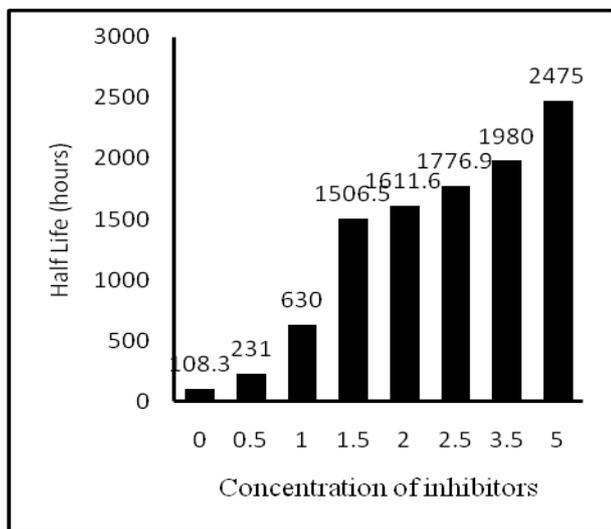
Fig.3: Half life of the corrosion of mild steel in 1M HCl without and with inhibitors
