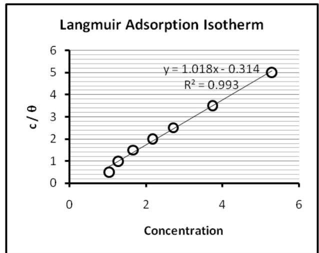
Fig-4: Langmuir Adsorption Isotherm
