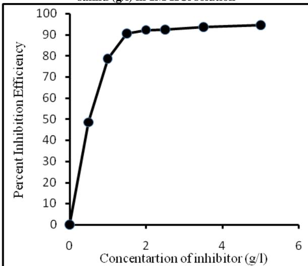
Fig-2: Variation of percent inhibition efficiency with concentration of Sakhu (g/l) in 1M HCl solution
