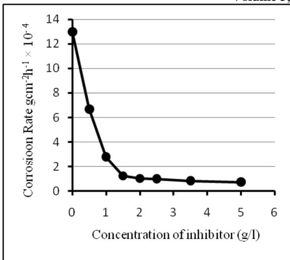
Fig-1: Variation of corrosion rate with concentration of sakhu (g/l) in 1M HCl solution
