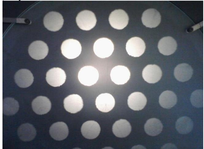
Fig.2 Observation of a laser drilled MPP after removal of the defaults (shavings and material particles). Observation obtained with a DELTRONIC profile projector (enlargement x10).
