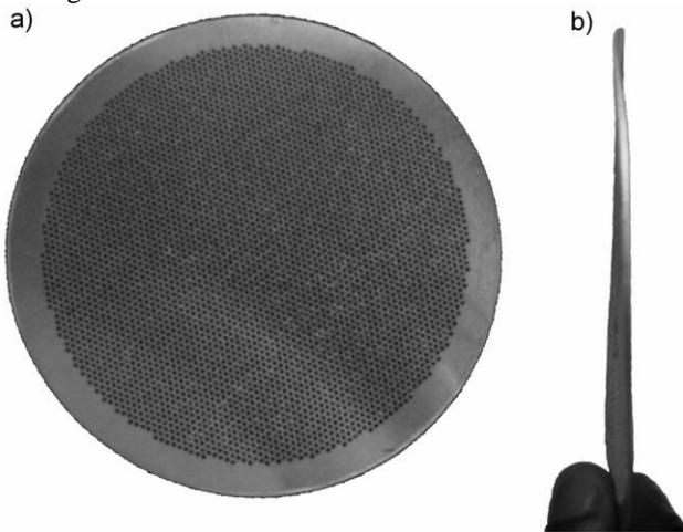
Fig.4 Picture of a Micro-perforated panel with 4300 holes of 0.9 mm in a circular plate of 100 mm diameter. The plate thickness is 1 mm and the distance between two consecutive holes is 1.3 mm. (a) front view; (b) profile view showing the resulted plate bending.
