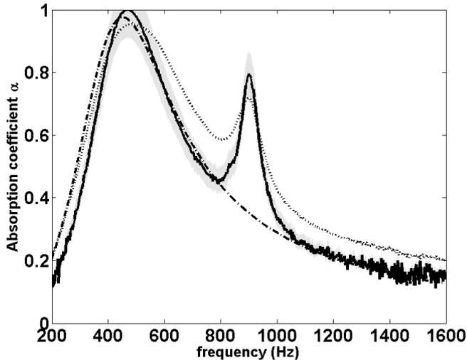
Fig.7 Absorption coefficient of sample MPP2. Air cavity depth of 50 mm. Solid line: measurement without the defaults; dotted line: rough measurement with defaults; dotted-dash line: simulation; Gray area: the confidence range.
