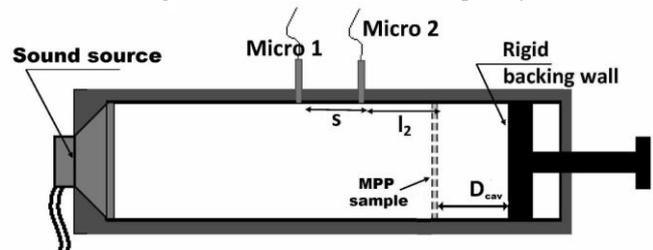
Fig.5 Impedance tube used for the measurement.
