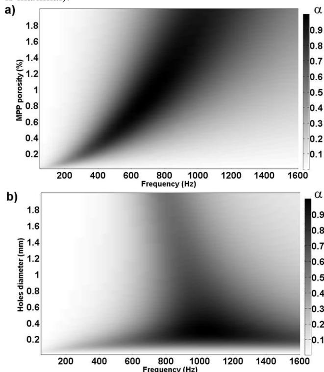
Fig.1 Simulated sound absorption coefficient as a function of the frequency. (a) Variation of MPP porosity (plate thickness of 1 mm, holes diameter of 0.5 mm and air cavity depth of 50 mm); (b) Variation of holes diameter (plate thickness of 1 mm, porosity of 1.94 % and air cavity depth of 50 mm).
