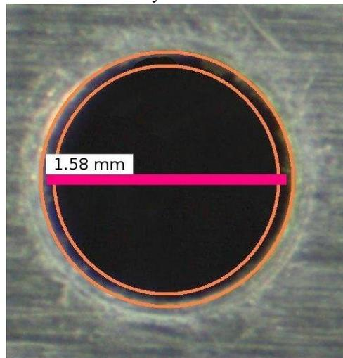
Fig.3 Picture of a single perforation laser drilled for a nominal diameter of 1.6 mm. Laser beam ray of 0.3 mm. Observation obtained with a digital microscope (x20).
