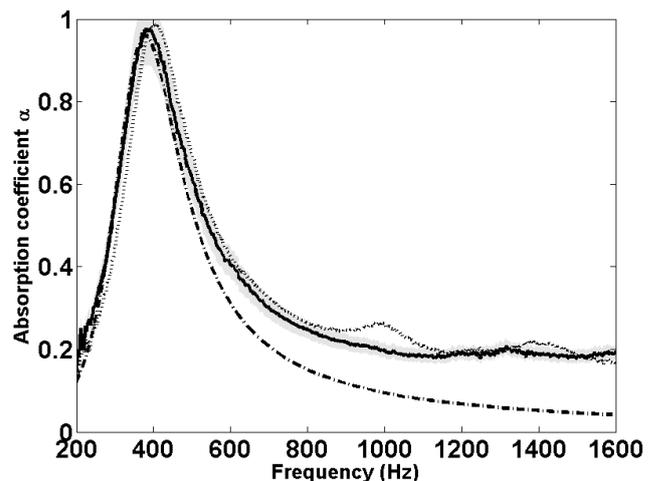
Fig.6 Absorption coefficient of sample MPP1. Air cavity depth of 50 mm. Solid line: measurement without the defaults; dotted line: rough measurement with defaults; dotted-dash line: simulation; Gray area: the confidence range.
