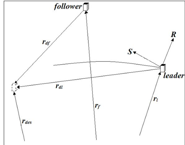
$$\begin{aligned} \ddot{x} &= -f_x + 2\omega\dot{y} + \dot{\omega}y + \left( \omega^2 - \frac{2\mu}{r_{tgt}^3} \right) x \\ \ddot{y} &= -f_y - 2\omega\dot{x} - \dot{\omega}x + \left( \omega^2 + \frac{\mu}{r_{tgt}^3} \right) y \\ \ddot{z} &= -f_z + \left( \frac{\mu}{r_{tgt}^3} \right) z \end{aligned} \quad (7)$$
