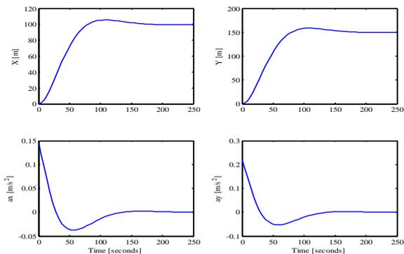
Fig 3: closed loop system response based on Lyapunov function
