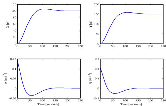
Fig 4: closed loop system response based on MPC algorithm
