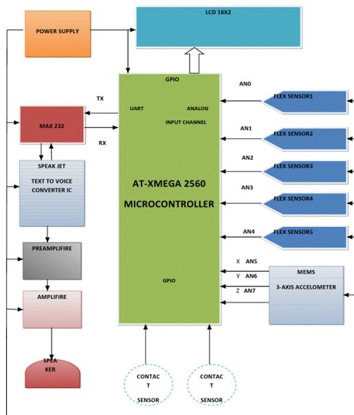
Fig 1: Block diagram of Automatic finger sign recognition
