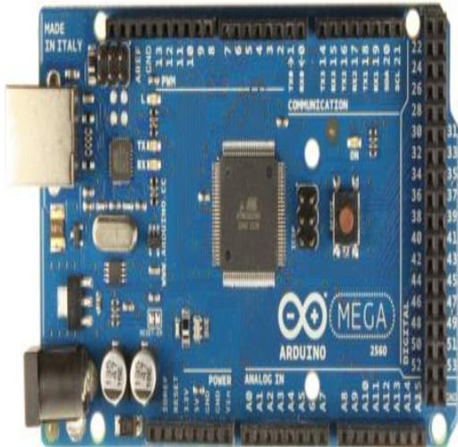
Fig 3: Microcontroller Arduino Mega 2560
