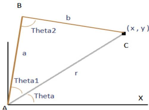
Fig.4. Arm axis movement
