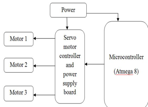
Fig.2. Block diagram 2D plotter
