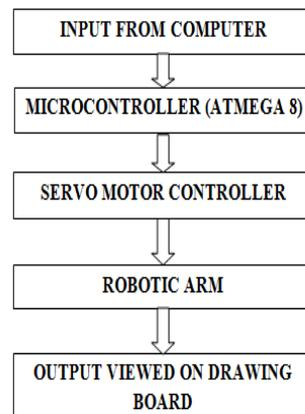
Fig.1. Flow chart of the Robotic 2D Plotter
