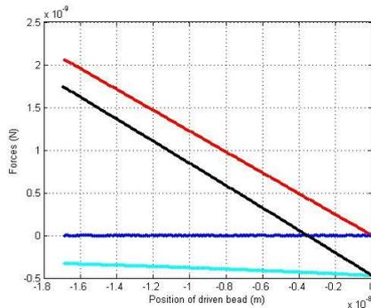
**Fig.7: Forces vs. position near tweezer center for case of  $I_0 = 1 \times 10^4 W/cm^2$ ,  $W_0 = 2 \mu m$ ,  $L_0 = -17 \mu m$**
