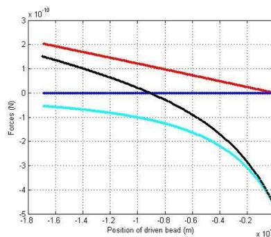
**Fig.6: Forces vs. position near tweezer center for case of  $I_0 = 1 \times 10^2 \text{ W/cm}^2$ ,  $W_0 = 2 \mu\text{m}$ ,  $L_0 = -17 \mu\text{m}$**
