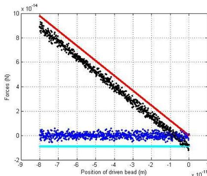
**Fig.8 Forces vs. position near tweezer center for case of  $I_0 = 1 \times 10^2 W/cm^2$ ,  $W_0 = 2 \mu m$ ,  $L_0 = -2 \mu m$**
