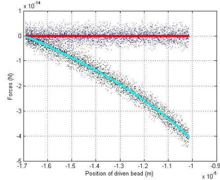
**Fig.2: Forces vs. position of driven bead at low stretched state: optical (red), Brownian (blue), elastic (cyan), total (black) for case of  $I_0 = 1 \times 10^2$  W/cm<sup>2</sup> and  $W_0 = 2 \mu m$ .**
