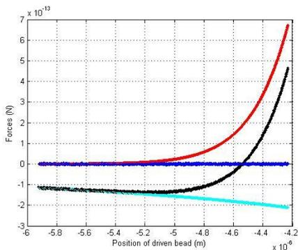
**Fig.3: Forces vs. position in region (6.0-4.2)  $\mu\text{m}$  for case of  $I_0 = 1 \times 10^2 \text{ W/cm}^2$  and  $W_0 = 2 \mu\text{m}$ .**
