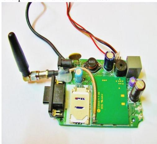
Fig. 2. Real view of GSM modem
