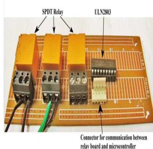
Fig. 3 SPDT relay board along with ULN 2803
