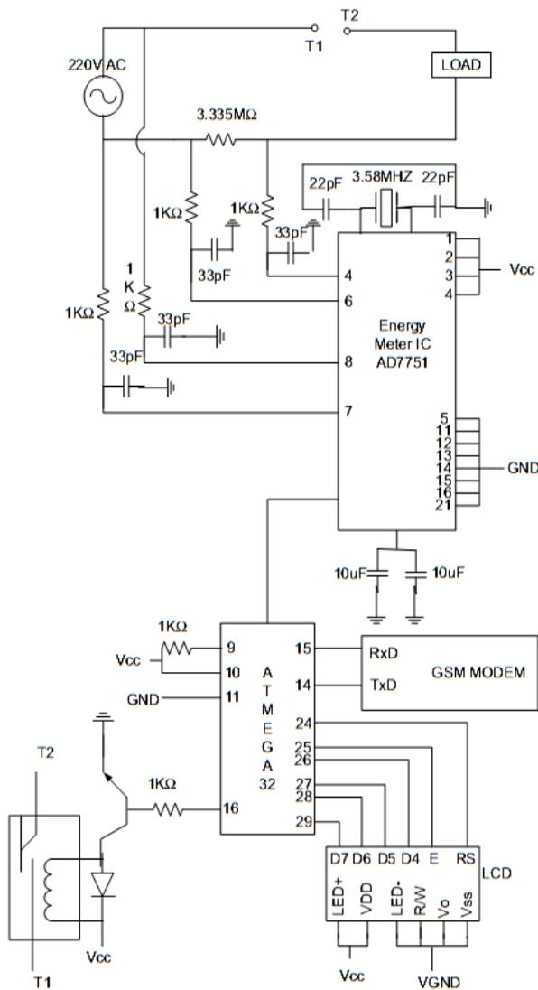
Fig. 5 Circuit layout of the energy meter
