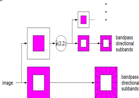
Fig-2The Contour let filter bank
