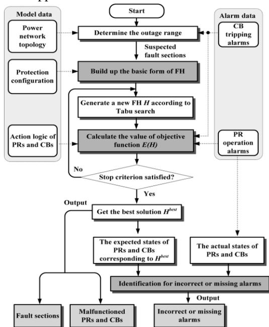
Fig. 1. Framework of the Developed Fault Diagnosis Method.
