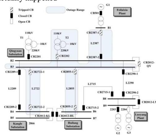
**Fig. 3. Power System Diagram Associated With the Fault Scenarios**
