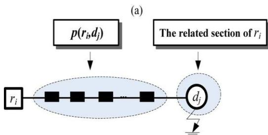
Fig-2: (a) Determination of the related section according to the protection zone of  $r_i$ . (b) Related path from  $r_i$  to  $d_k$ .
