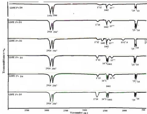
Fig.8: Comparison FTIR Spectra of LDPE- 1% Fe MFA in Presence One To Five Day (D0-D5) UV Exposure
