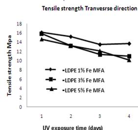
**Fig .3 Effect Of MFA on Tensile Strength of LDPE-Fe MFA (Transverse Direction)**
