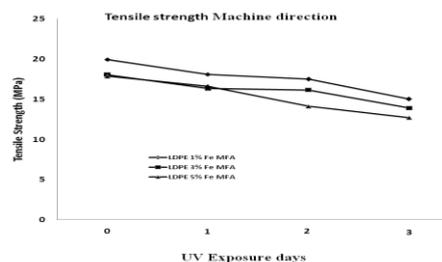
**Fig .2 Effect Of MFA on Tensile Strength of LDPE-Fe MFA (Machine Direction)**
