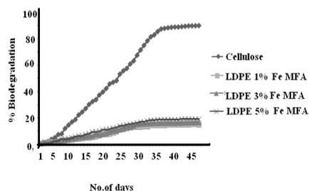
**Fig. 14: Bio-Degradation Curve of LDPE Films In Presence Of 1%, 3 %, And 5% MFA**
