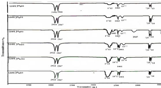
Fig.9: Comparison FTIR Spectra of LDPE- 3% Fe MFA in Presence of Five Day (D0-D5) UV Exposure
