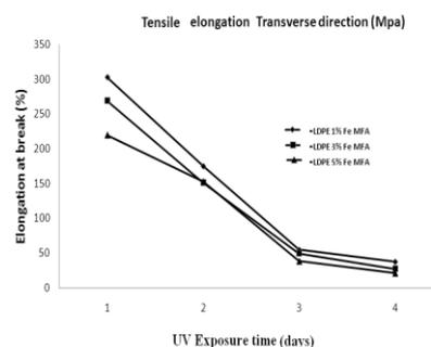
**Fig. 5 Effect of MFA on elongation of LDPE-Fe MFA (Transverse Direction)**
