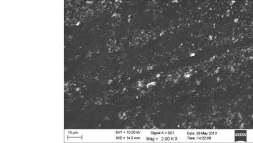
Fig.12: Effect of MFA on Morphology 5% LDPE -Fe MFA without UV exposure.
