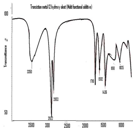
**Fig .6: FTIR spectra of MFA (Ferrous 12 hydroxy oleate)**
