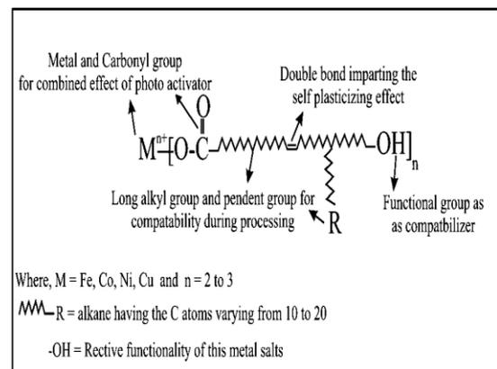
Fig. 1: Generic Structure of Multi Functional Additive (MFA)
