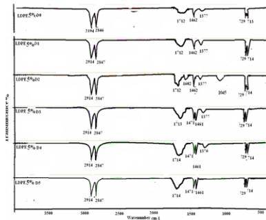
Fig.10: Comparison FTIR Spectra of LDPE- 5% Fe MFA in Presence of Five Day (D0-D5) UV Exposure
